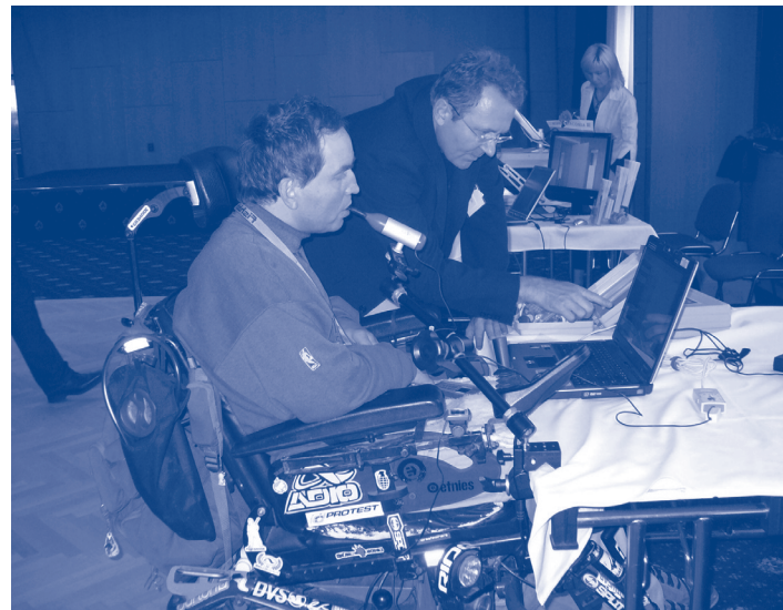
Mr. Miloš is able to work at the computer, thanks to "IntegraMouse," which makes it possible for him to activate all of the available functions of a standard computer mouse with his mouth. Clicking on the left or right button is produced by changing the force of the air in the mouth cavity and thus in the mouthpiece.
